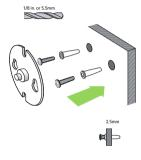
Align base with plate and screw on camera post.
