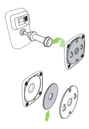
Attach screws to wall and hang plate onto screws.
