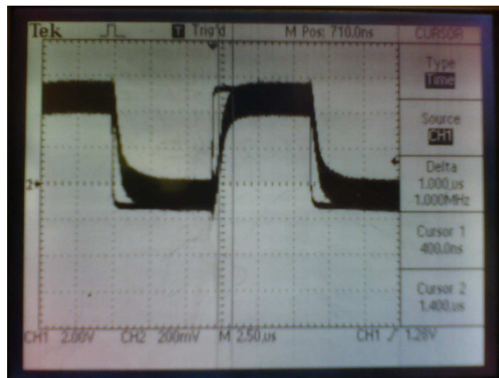
Figure 5-2 - TIA Test Output with Oscillations
