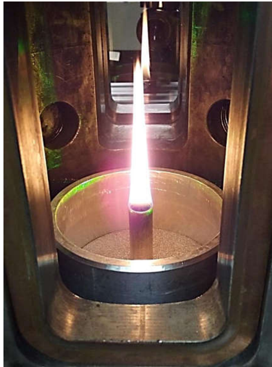
Figure 10. Gülder's burner laminar ethylene diffusion flame in the Soot Lab
