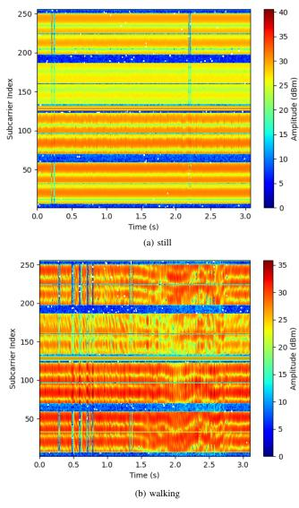
Fig. 3: Comparison of still and walking CSI readings.
