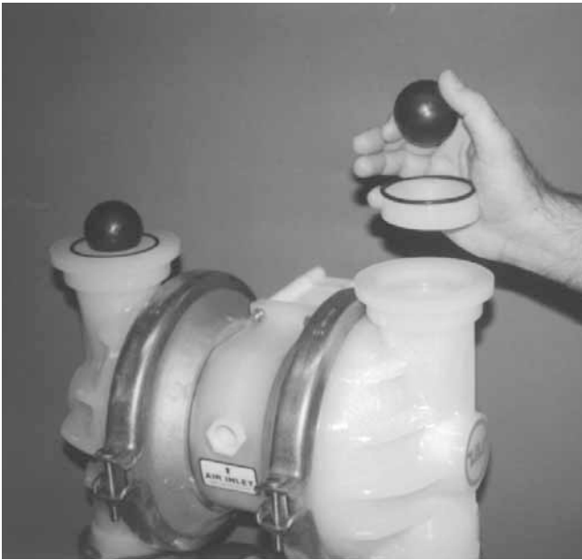
Step 4. Figure 4 Remove the discharge valve balls and seats ( Figure 4 ) from the liquid chambers and inspect for nicks, gouges, chemical attack or abrasive wear. Replace worn parts with genuine Wilden parts for reliable performance.
