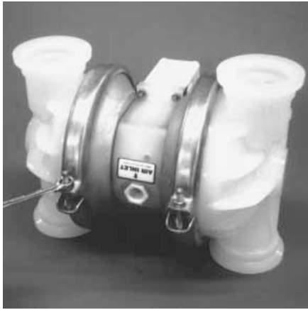
Step 9. Figure 9 Remove one set of large clamp bands which secure one liquid chamber to the center section. ( Figure 9 )
