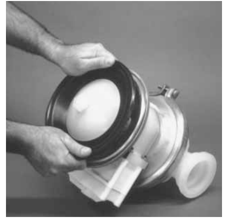
Step 11. Figure 11 Using an adjustable wrench, or by rotating the diaphragm by hand, remove the diaphragm assembly. ( Figure 11 )
