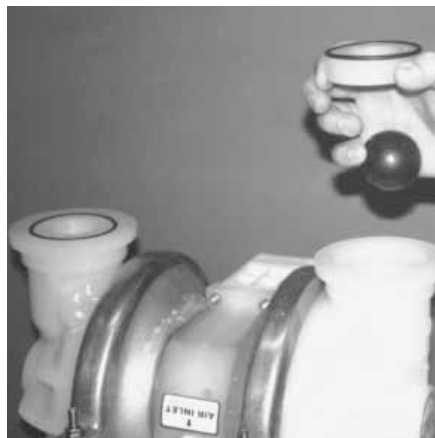
Step 7. Figure 7 Remove valve seats and valve balls for inspection. Replace if necessary. ( Figure 7 )
