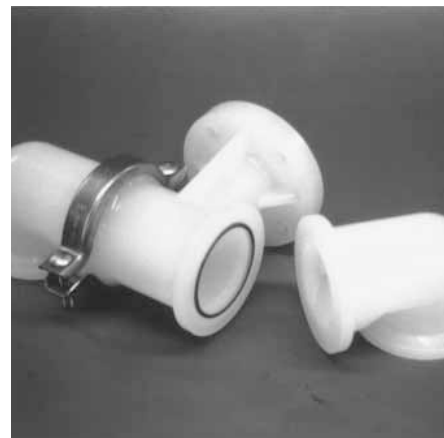
Step 8. Figure 8 Remove small manifold clamp bands to inspect manifold O-rings. ( Figure 8 )
