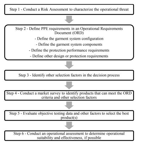
Figure 4-1. WLFF PPE Selection Process Flow Chart
