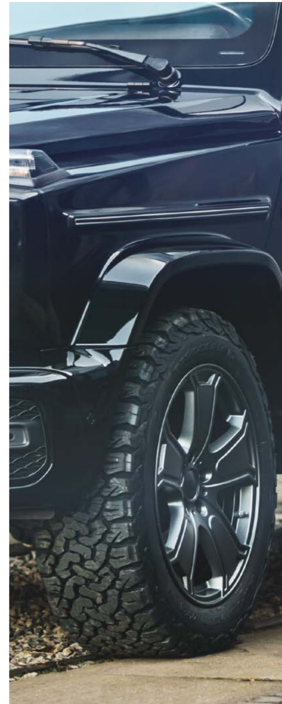
20" rough profile offroad tires on grey mat painted heavy duty wheels with runflat system (50 km at 50 km/h)
