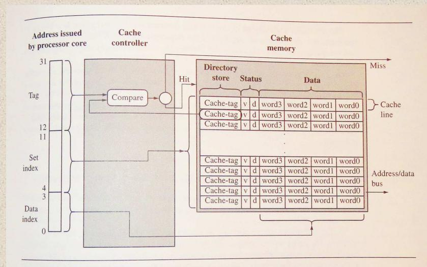
Figure 12.4 A 4 KB cache consisting of 256 cache lines of four 32-bit words.
