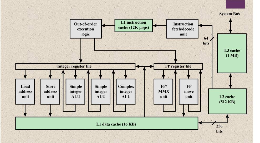
Figure 4.18 Pentium 4 Block Diagram
