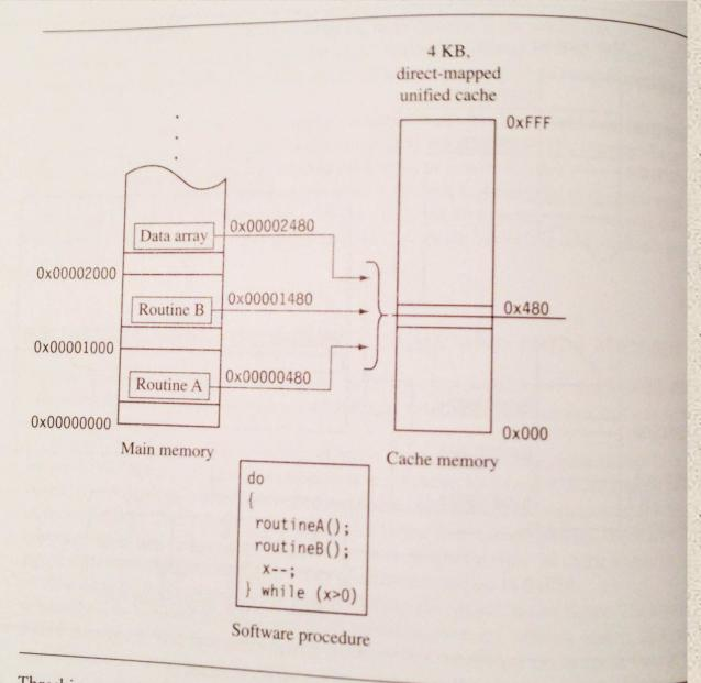
Figure 12.6 Thrashing: two functions replacing each other in a direct-mapped cache.
