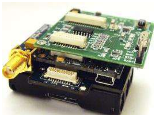
ISM400 board stacked on Imote2
