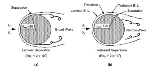
Figure 5: Flow Field Elements about a Cylinder (Sakamoto)  $\theta = degree \ of \ flow \ separation$
