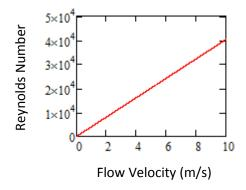
Figure 2: Reynolds Number versus Flow Velocity (m/s)
