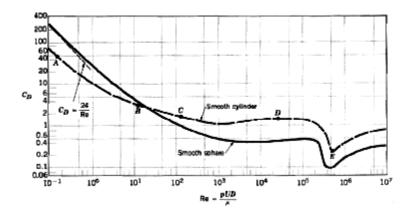
Figure 6: Drag Coefficient for a Smooth Cylinder as a Function of Reynolds Number (Drag of Blunt Bodies...")
