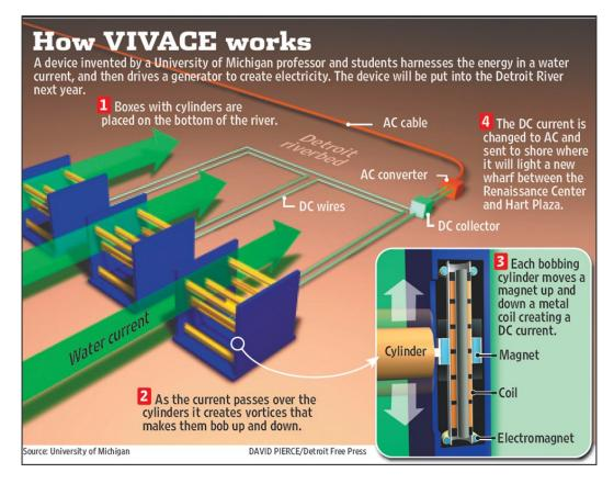
Figure 14: How VIVACE Works (Vortex)
