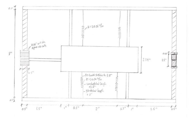
Figure 15: Sketch of Initial Design, Front View
