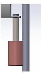
Figure 29: New Magnet and Coil Assembly, with Magnetic Sheilding Foil
