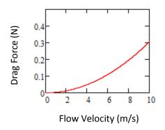
Figure 18: Drag Force (N) versus Flow Velocity (m/s)
