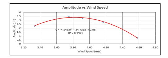
Figure 25: Graph of Measured Amplitudes over Range of Flow Velocities
