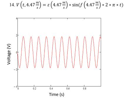
Figure 23: Theoretical Voltage Output (V) over Time (s) *(for the 100 Turn Coil System Explained Above)*
