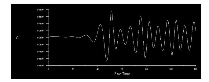
Figure 7: Lift Coefficient of a Cylinder as a Function of Flow Time (Distler)
