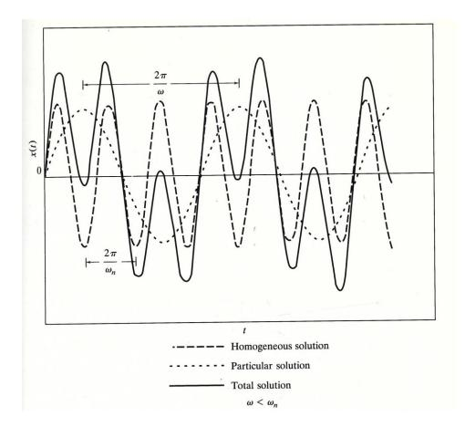
Figure 10: Displacement versus Time for Situation Where  $\omega < \omega_n$  (Kelly)
