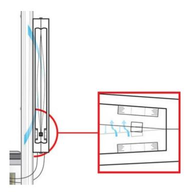
Figure 13: Sketch of Windbelt, Depicting Membrane, Magnets, and Coils (Ward) Frayne's design uses a taunt membrane, made of Mylar-coated taffeta, and a pair of magnets which oscillate between metal coils (Figure 13). The potential cost for Frayne's device is a few dollars. He hopes it can replace kerosene lamps in Haitian homes – instead of the flammable kerosene lamps, Haitian's could instead use LED lamps powered by the Windbelt.
