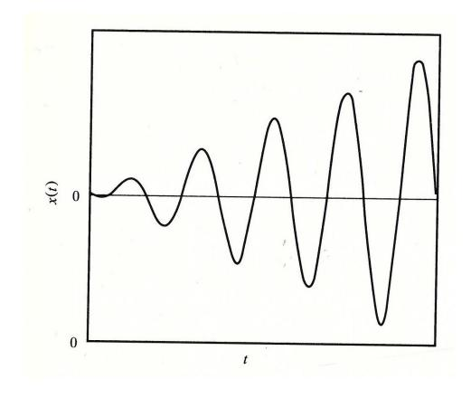
Figure 11: Displacement versus Time for Situation Where  $\omega = \omega_n$  (Kelly)
