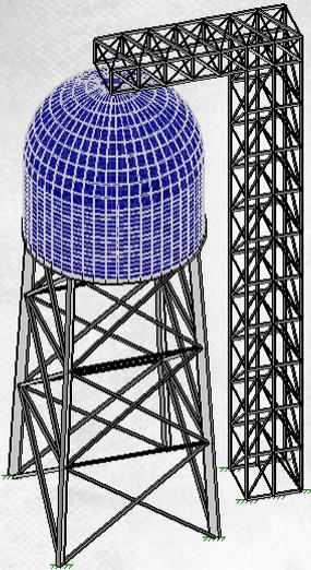
Tank and Legs:  $n = 8.4 \text{ Hz}$  (Rigid)  $G = 0.85$
