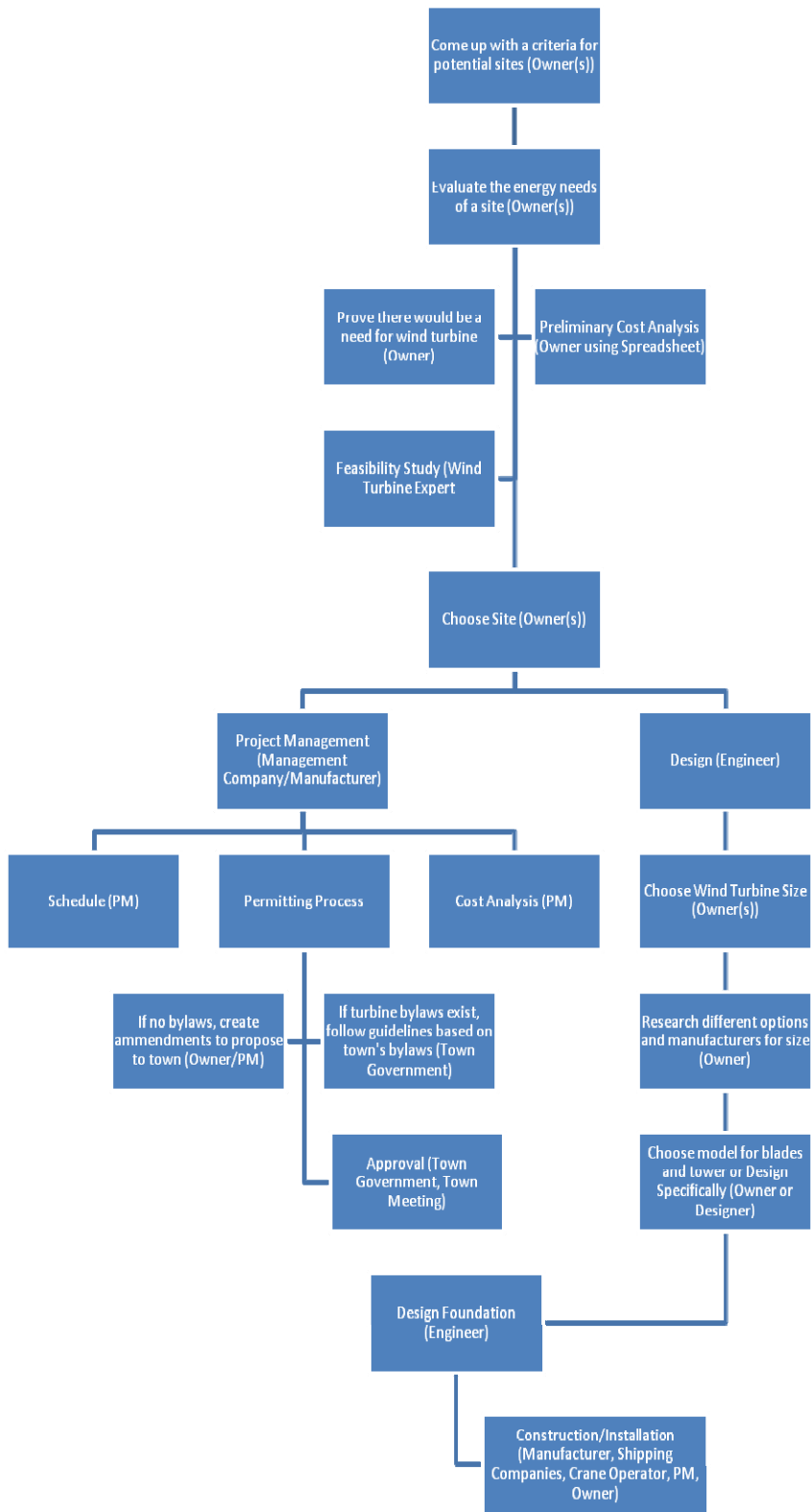
Figure 3: Planning Process of Installing a Wind Turbine
