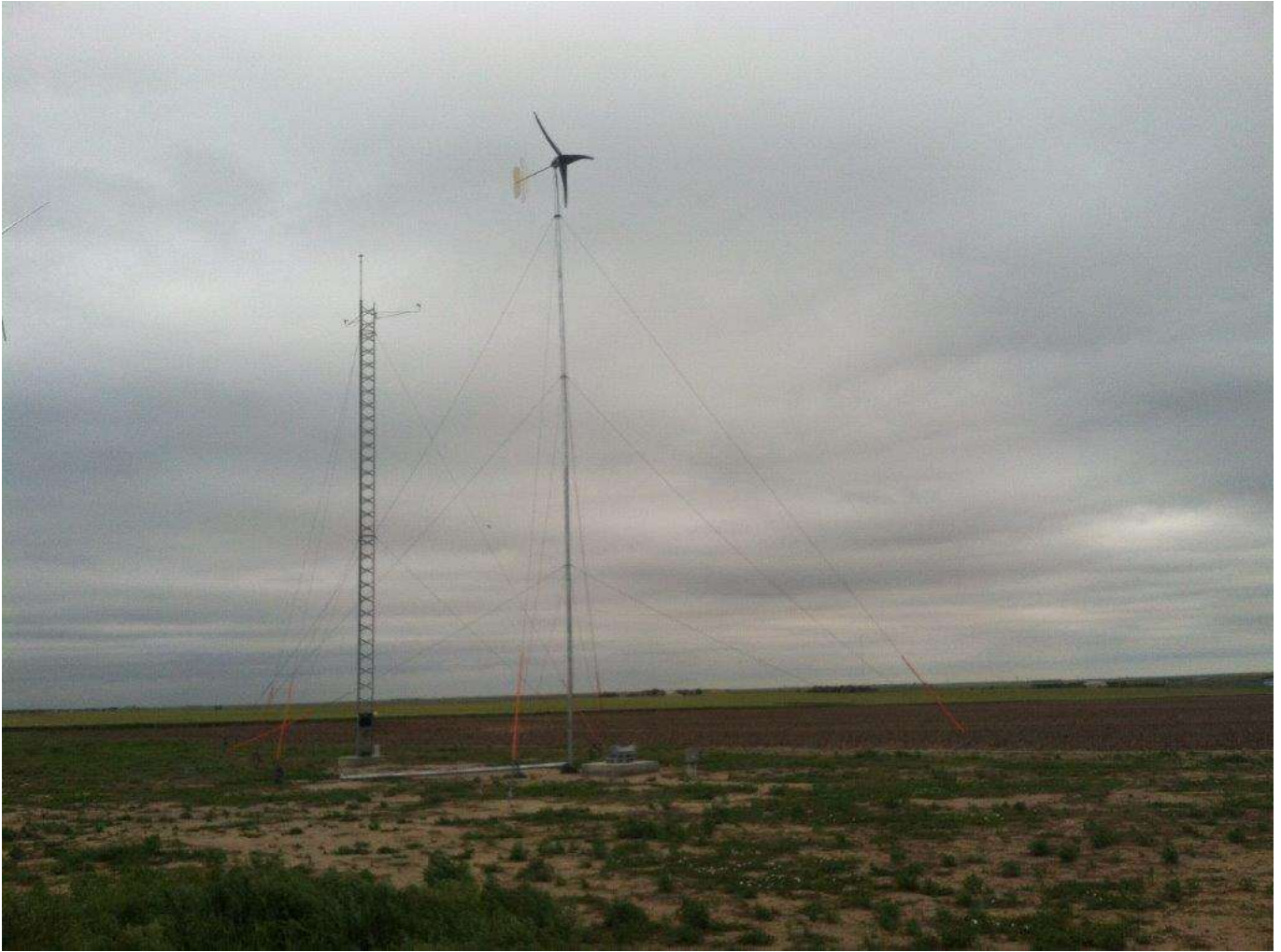
Figure 1. Pika T701 turbine installed at High Plains Small Wind Test Center, met tower behind; view is towards the northwest.
