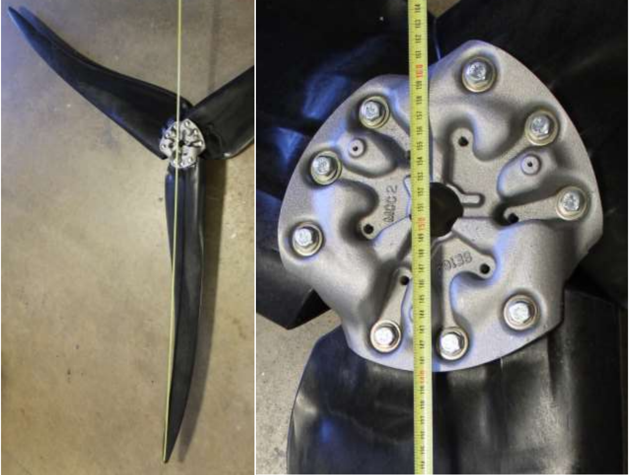
Figure 2. Pika T701 rotor showing radius measurement
