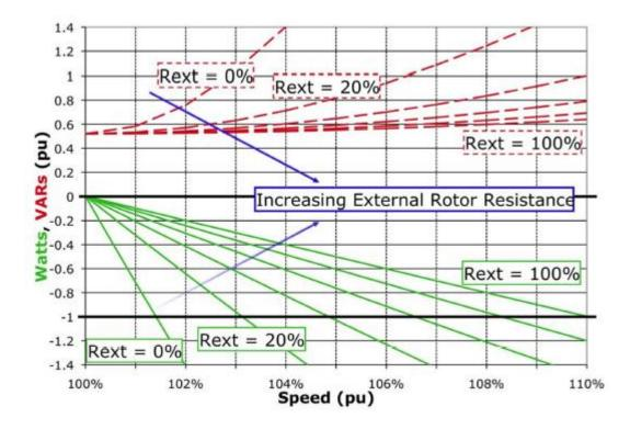
Variable Speed with Partial Power Electronics Conversion (Type3)
