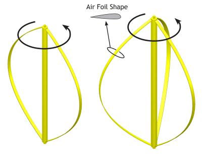
The Darrieus turbine is not self starting. It needs to start turbing before the wind will begin rotating it.
