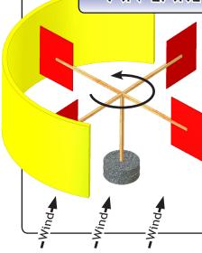
The Persian windmill was used around 1000 b.c. to turn a grindstone. It is the oldest known windmill design. The machine works by blocking the wind blowing on  $\frac{1}{2}$  of its sails. The sails exposed to the wind are pushed downwind due to drag, causing the windmill to rotate.
