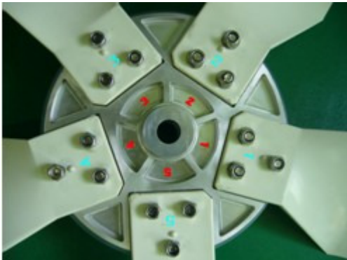
5、 SAME AS STEP THREE, ASSURE THE BLADE NO. AND HUB NO. MATCH.
