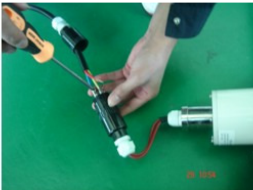
1、 CONECTTHE THREE FAHSE WIRE WITH WIND TURBINE THREE PHASE WIRE
