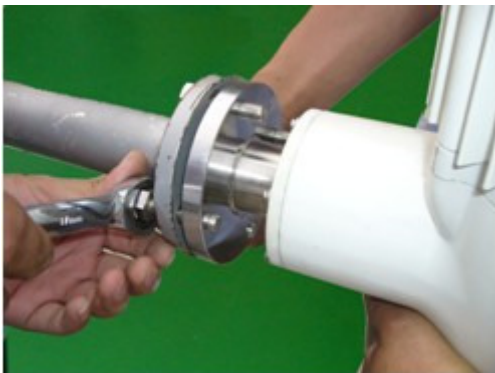
5、 ATTACHED THE FLANGE AND TOWER WITH LOCKNUTS
