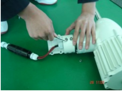
3、 ATTACH THE UPPER COVER AND REDUCING JOINT THEN FASTERN BY NUTS
