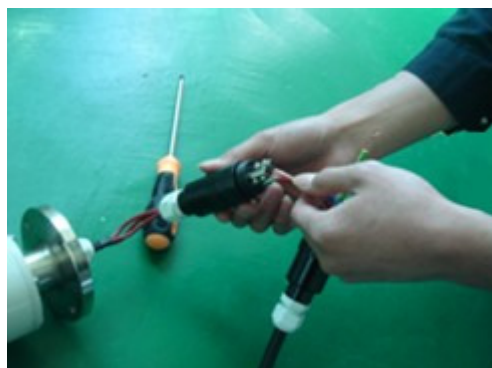
2、 PULL OUT THE CABLE COVER AND CONEECT THE CABLE'S THREE FAHSE WIRE WITH WIND TURBINE THREE PHASE WIRE
