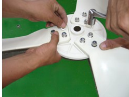
4、 FASTERN THE BLADES ON HUB WITH STUD & NUTS
