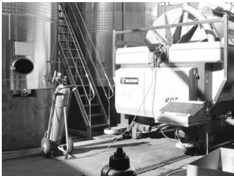
Fig. 12.3 Inert gas injected into tank press
