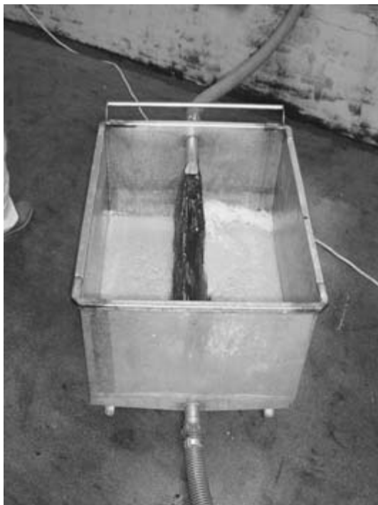
Fig. 12.6 Aeration during pump over
