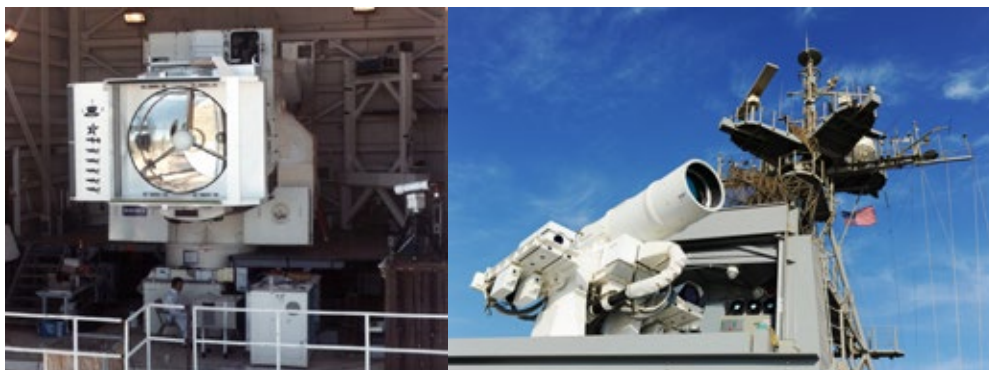
FIGURE 24: BEAM DIRECTORS FOR THE MIRACL LASER AND LAWS DEPLOYED ON THE USS PONCE
