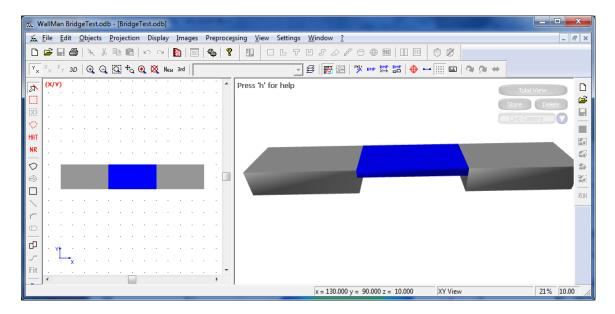
The new objects are considered in ProMan when using the urban propagation models (DPM, IRT). Accordingly the opening under the bridge is considered for the wave propagation. Furthermore the predictions are performed also in the area below the bridge.
