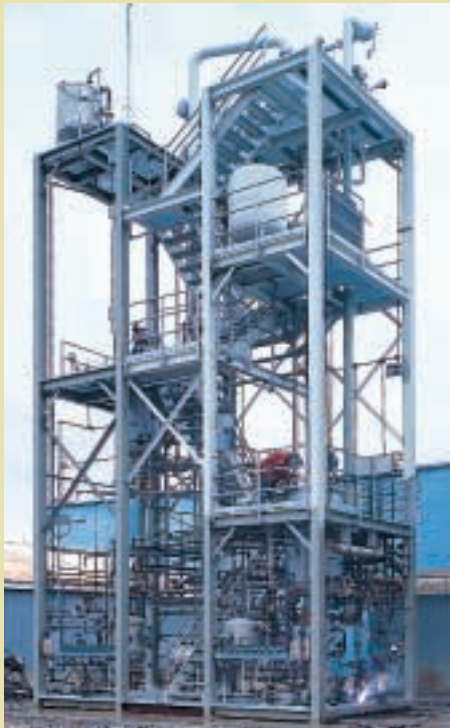
Multi-stage WFE skid-mounted system
