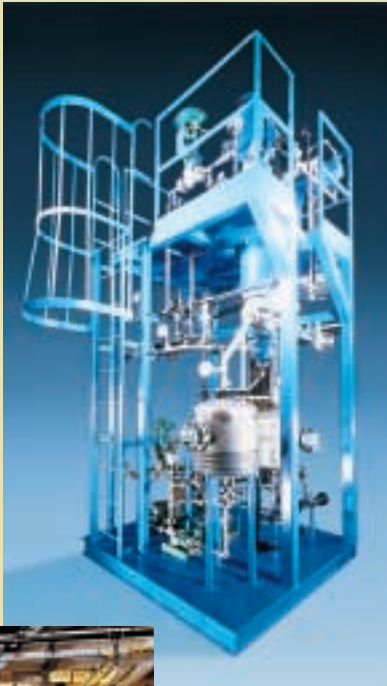
Skid-mounted 8.8 sq. ft. WFE for solvent recovery
