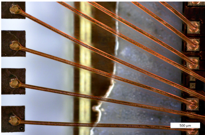
Figure 2. EDF image of wire loops between ball bonds and wedge bonds. 5x objective. 101x mag.
