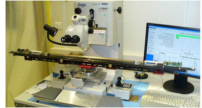
Pull Tester Station
