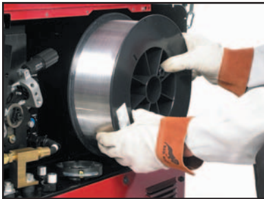
Easy Load Wire Compartment
