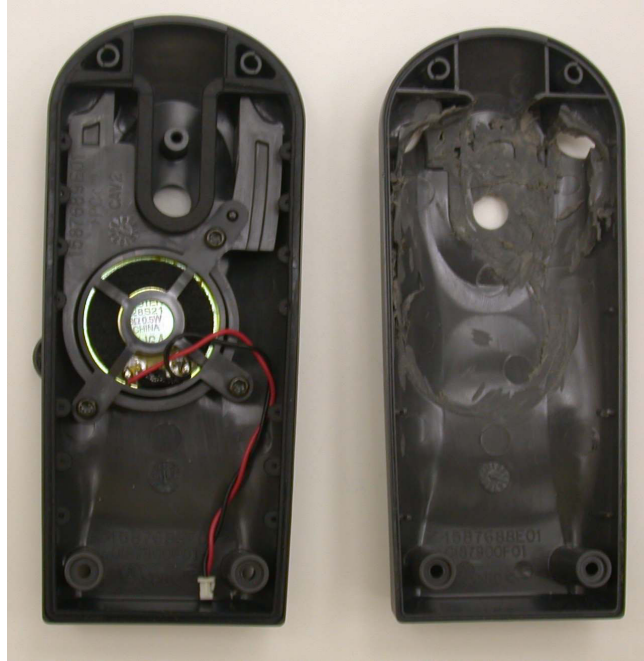
Figure 7.3: Side by Side View of Original Motorola Stand and Hollowed-out Stand
