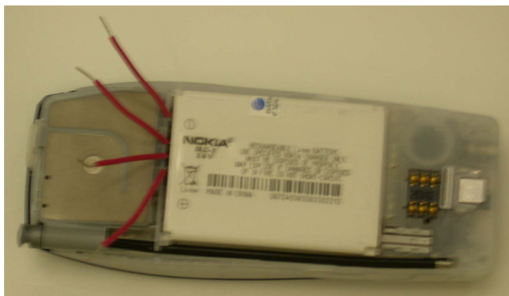
Figure 6.10: Battery In Nokia Phone with External Leads
