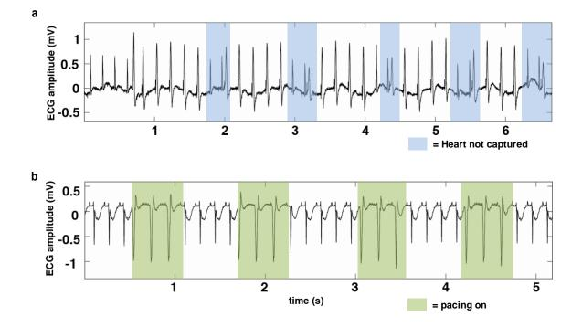
**Supplementary Figure 9** Additional in vivo pacing functionality. (a) Inconsistent pacing is not able to fully capture the heart after Day 6 in vivo pacing but device is still able to deliver electrical stimuli. (b) On/off settings of pacemaker is easily toggled in the order of seconds.
