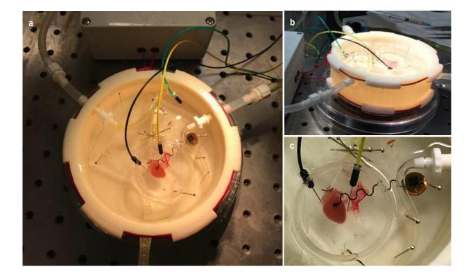
Supplementary Figure 7 Langendorff-perfused heart system set-up. (a) NeuroLux pacing set-up with custom chamber for Langendorff-perfused heart. (b) Side view of customized wireless power transfer chamber with NeuroLux pacing system. (c) Placement of device onto anterior epicardial surface of a mouse heart.
