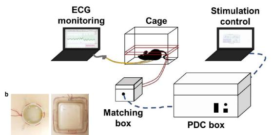
**Supplementary Figure 6** In vivo stimulation system set-up. (a) Full system set-up. (b) Modular antenna allows for customized power transfer chambers.
