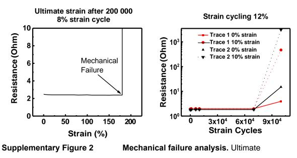
electrical and Mechanical strain of electrodes and cycling above elastic limit.
