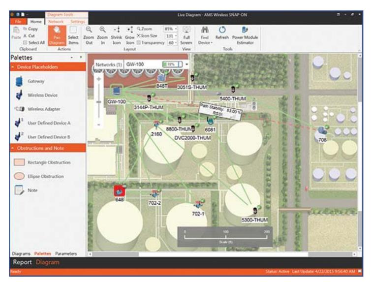
Figure 3. Process plant plot plans can be uploaded to Emerson's AMS Wireless SNAP-ON software, and the wireless network can then be overlaid on these plans. The software can be used to check design validity, and to monitor networks after installation. (Courtesy of Emerson Process Management)
