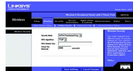
Figure 5-12: Wireless Tab - Wireless Security (WPA-Preshared Key)
