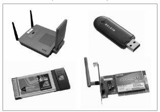
Figure 1-8 Access point (upper-left) and wireless NICs
