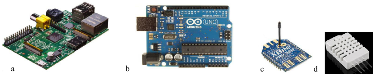
Fig. 2. (a) Raspberry Pi Model B; (b) Arduino UNO R3; (c) XBee Pro S2B; (d) RHT03 Temperature and humidity sensor.
