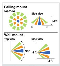
Fresnel lenses molded into the faceted cover of the sensor broaden the sensing area, both horizontally and vertically.
