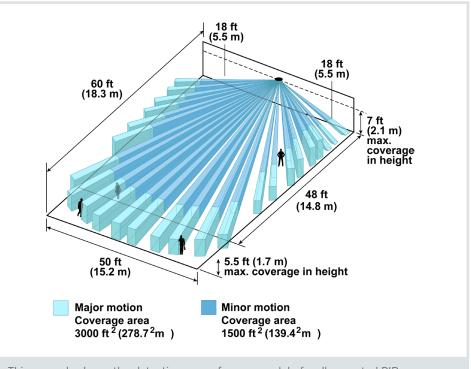
This example shows the detection range for one model of wall-mounted PIR sensors.
