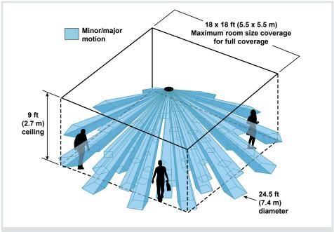
This example shows the detection range for one model of ceiling-mounted PIR sensors.
