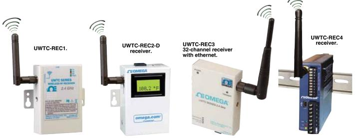
UWTC-REC1 will receive data from up to 48 transmitters and is powered directly by the USB connection on your computer (no analog output provided). UWTC-REC2-D will receive data from up to 48 transmitters. This model provides a displayed reading and a retransmitted, hard wired analog output for 1 user selected transmitter in your system. Requires DC power adaptor (included).
