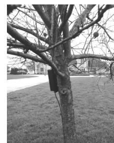
DA-611TO transmitter box in a tree for greater range
