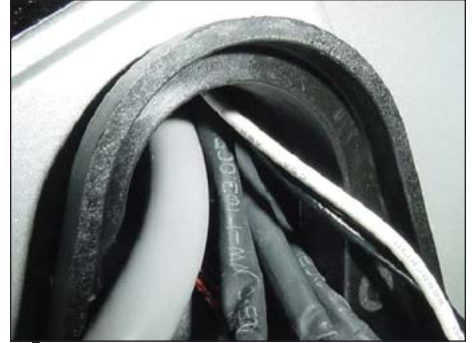
Opening for wires and harnesses as viewed from the other side of the Motor Arm Assembly.
