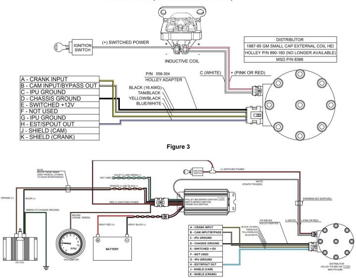
HOLLEY EFI TO GM HEI IGNITION - USING COMPUTER CONTROLLED DISTRIBUTOR, EXTERNAL COIL (ECU CONTROLLING TIMING)
