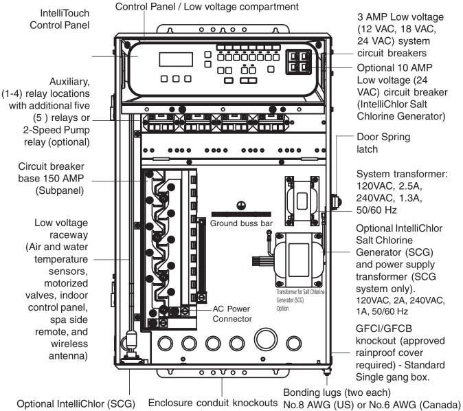
Optional IntelliChlor (SCG) cell connector socket
