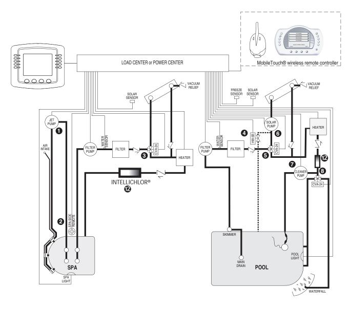
Recommended Hydraulic Schematic for Dual Equipment System
