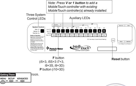
4. From the MobileTouch controller Advanced screen, press the **lower buttons 2 and 4 at the same time**. The Service Personnel screen will be displayed.
