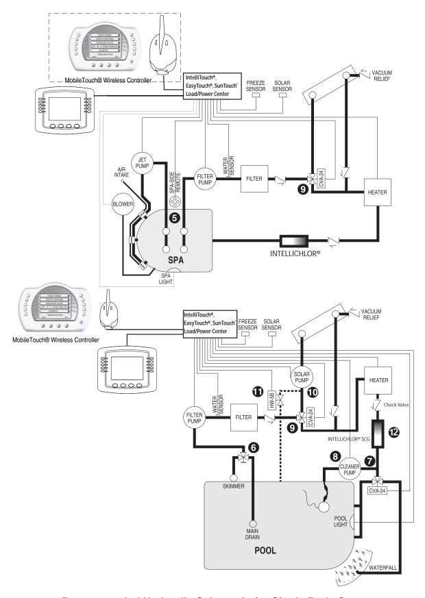
Recommended Hydraulic Schematic for Single Body System
