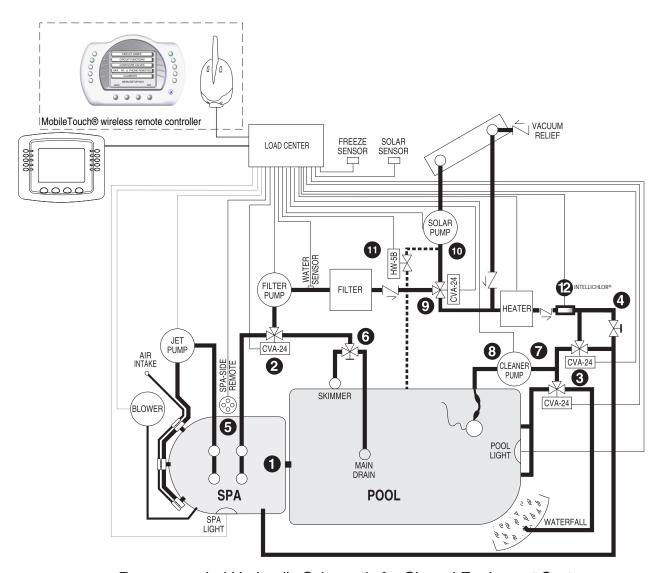
Recommended Hydraulic Schematic for Shared Equipment System
