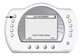
6. Note: Before pressing the "Lock On Address" move at least 20 to 30 feet away from the transceiver. Press the button next to LOCK ON ADDRESS to assign a unique frequency for the MobileTouch controller to avoid inference from other wireless devices within range of the MobileTouch transceiver.
