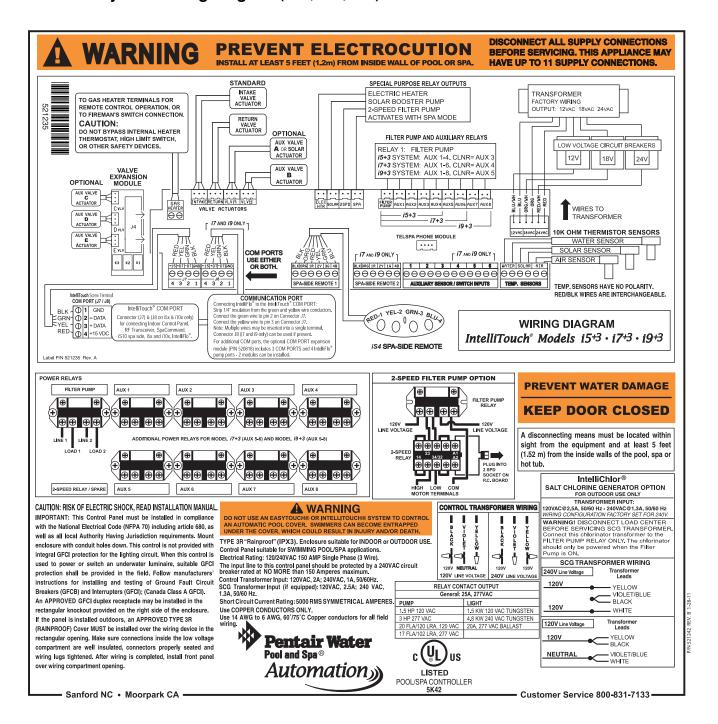
**IntelliTouch System Wiring Diagram**
