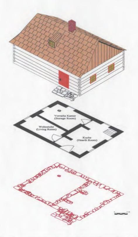
**Figure 59:** A conjectural reconstruction of the Hoffnungsthal mission house. For clarity the east dormer window is omitted.
