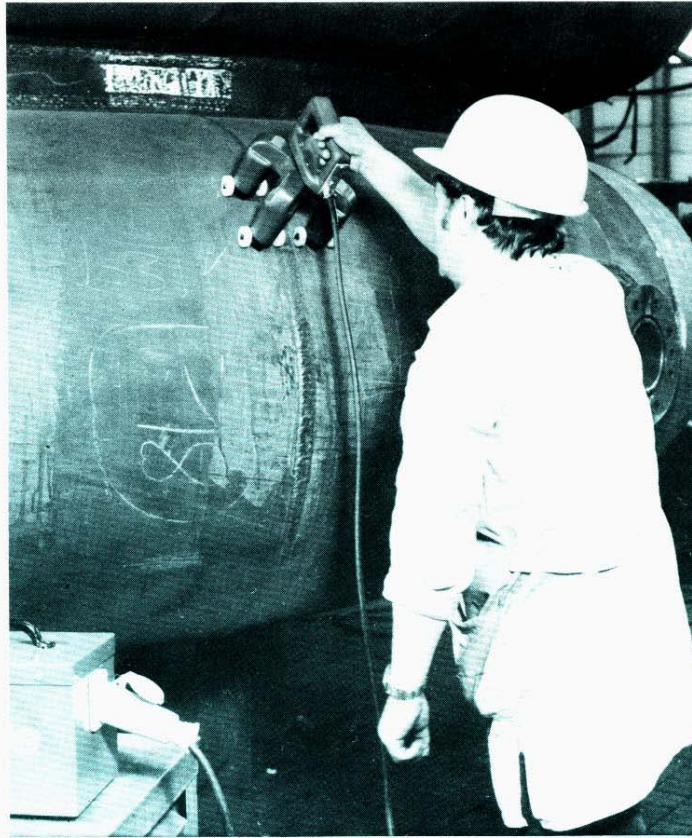
Inspector magnetizes weld with cross yoke, inducing magnetic fields in two directions. Magnetic particles reveal transverse and longitudinal discontinuities.
