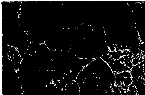
Figure 9a.- Overheat zone of a non-conductive carbon steel; ferrite as net work and Widmannstatten needles.
