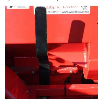
**Hydraulic wedge** – is adjusted with a lever on the control panel. "Feathering" this lever allows for more subtle adjustments.
