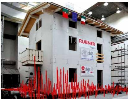
Among other programmes, Rubner has executed extensive research works at the University of Trient and has participated in the inter-university research project "Series", which comprised vibration table tests in real-life scale. This extensive research work allowed to develop and test company-specific construction details, which have provided the basis for complex and architectonically demanding timber constructions in earthquake-endangered regions.
