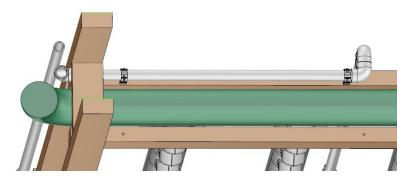
Figure 3 - View from underneath showing 1" Quick Latch on Rail
