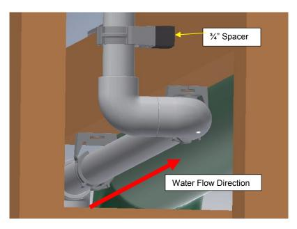
Figure 12 -- 1" Supply Line under Rail in the middle of the tower
