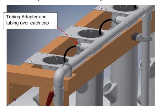
On the left side of the stand, the pipe is terminated in a cap.
