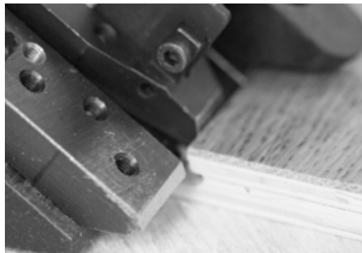
Fig. 13 Pushed in to the groove = correct position
