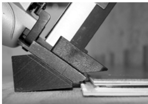
Fig. 9 Nail gun lifted over the locking element
