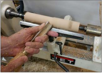
**7. Handle** — *Use the spindle roughing gouge to round the handle blank.*
