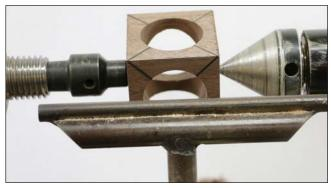
**4. Mount between centers** — The cup drive in the headstock will allow the blank to slip if there should be a catch or too much force while cutting.
