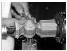
**1. Round the ball** after making a second chucking tenon on the tailstock end.
