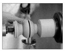
**3. Part** the ball using a narrow tool.
