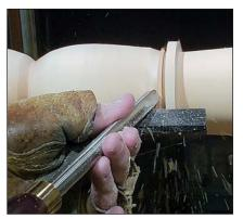
**8. Tight spot.** Detail gouge slices down to a tight corner.
