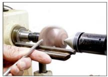
**8. Cut downhill** — Continue shaping the right and left sides to round the cube. Remember to cut from the largest-to-smallest diameter, cutting downhill toward the tailstock or cup drive.
