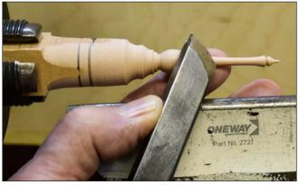
**12. Underhand grip** — Detail the finial with a spindle roughing gouge, 3/8" (10mm) spindle gouge, and a small curved skew, or equivalent carbide tools. With the blank in pin jaws, you can use an underhand grip to steady the thin spindle; if you are a novice, uncomfortable, or do not have the correct chuck jaws, use the tailstock for support.
