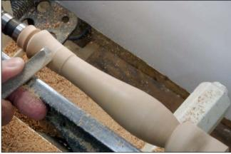
**11. Finishing cut** — The red oak handle takes a nice texture straight from the skew chisel.
