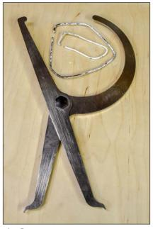
**6. Gauges** — As you hollow, check the wall thickness with a thickness caliper or a simple gauge bent from coat-hanger wire.
