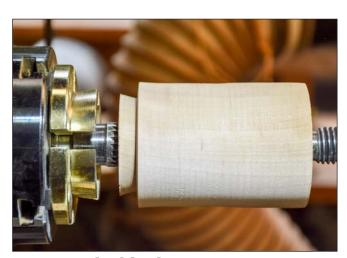
**1. Tenon the blank** — Turn between centers until the block is round and make a chucking tenon on one end.
