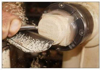
**2. Create a tenon** — Start with the roof, creating a tenon to fit the chuck jaws on what will be the top of the roof.
