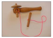
**Pull-string top**, left, loaded and ready to go. Top right, turned handle and spinning top. Below right, fit the top, insert the string and rewind
