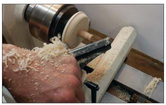
**5. Remount** — Reverse the workpiece in the chuck to turn the bottom side and spinner point.
