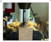
A drill press offers an alternative to boring on the lathe. Secure the blank in something other than your hand.
