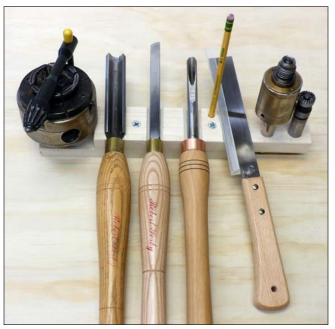
**1. Tools** — From left, scroll chuck, 3/4" (20mm) spindle roughing gouge, 1/2" (12mm) skew, 3/8" (10mm) bowl gouge, froe for splitting straightgrained spindle blank from sawn hardwood board, live center, and drive center.
