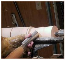
**6. Shaping.** The large spindle roughing gouge removes material accurately and quickly.
