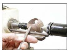
**7. Rub the bevel** — Start the cut with the bevel on the wood. Check tool presentation with the lathe off and you will be less likely to get a catch.
