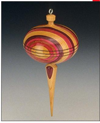
**Part, hollow and glue** — Colorwood ball was parted along the central burn line so the halves could be hollowed like two small bowls, then it was glued back together. Integral finial was turned last.
