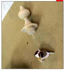
**22. Drill the tenon** — to receive the wire holding the perch.
