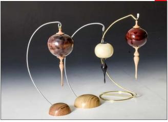
**17. Stands** — The stands can be purchased online or you can make your own, using steel wire from the hardware store. My wire came coiled in a tight circle about 6" (15cm) in diameter, so I cut about two-thirds of the circle and bent the hanging loop in one end. For the base, turn a block, bore a hole at an angle the size of the wire and attach. You can alter the height for different length ornaments by gently pulling or pushing.
