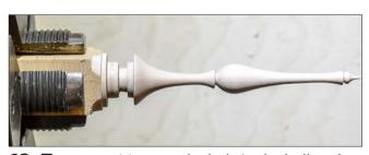
**13. Tenon** — Measure the hole in the ball and turn a small plug tenon before parting off. There's enough wood left in the chuck for the top finial.
