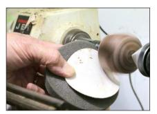
**9. Sand** — Start with 100 grit and move through 400 grit. A foam pad backing the abrasive will save your fingers and sand the corners evenly.
