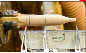
**11. Finial blank** — Choose dry, straight-grain, knot-free wood, big enough once it's rounded to cover the flats on the ball. Stick with the rule of thirds to design the finial elements and details. Mark the mounting tenon and major divisions on the wood.
