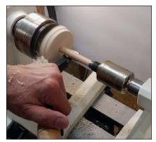
**3. Turning the top** — *With the bowl gouge, cut into the face and toward the headstock.*
