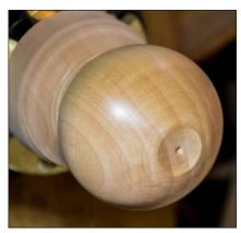
**3. Flat** — Make a flat spot for the finial, much easier than trying to fit it to the curve of the globe. Cut a dimple to give the drill bit a start.
