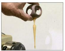
**17. Check the fit** — The tenon should fit the 3/8" hole drilled in the cube.
