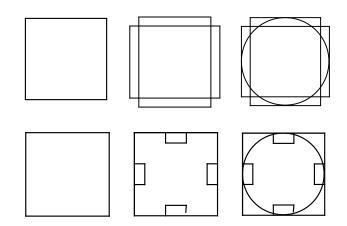
Mount the glued assembly between centers and turn round, without removing any unnecessary wood. Cut a tenon on the waste end of the blank, rechuck, bore 5/8" (2cm) for hollowing, and form the ball.
