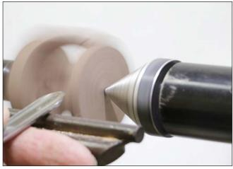
**5. Round the corners** — The blank is small and you will be cutting air a good part of the time, so a lathe speed of at least 1200 rpm improves the cut surface. Round off the corners to make a sphere using a 3/8" (10mm) spindle gouge.
