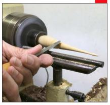
**14. Shape the "onion"**– Smooth the long transition from the tip, then shape a bulb. Finials are developed by completing elements from tail end-to-headstock.
