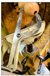
**7. Measure** — With the caliper points touching the wood inside and out, the free end shows thickness. Make hardwood about 1/8" (3mm) thick; lightweight woods can be thicker.
