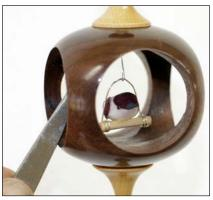
**23. Measure the wire** – Fully insert the wire into the hole in the top finial to see that the bird sits where you want it. Clip or redo as needed.
