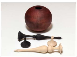
**16. Assembly** — There are many surface treatments you can apply to enhance the globe, including pyrography, paint and dye, or leave it plain. This one is dyed red, with two finials, one colored with black shoe dye, which gives it the look of ebony when finished. For assembly, use epoxy or regular wood glue, not super glue, because if it runs it can ruin your finished work.
