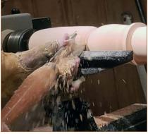
**7. Detailing.** Wing of roughing gouge cuts the quirk between body and head.
