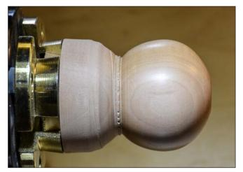
**2. Rough ball** — Use the spindle gouge to shape the sphere, but don't make the neck smaller than the chucking tenon.
