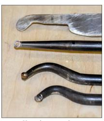
**5. Hollowing tools** — A simple steel scraper, top, can handle the hollowing. I like the new carbide-cup tools. After boring the starter hole, use the straight tool to open it up and make room for the bent tools.
