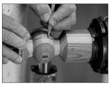
**2. Reference line** across the high point will help reassemble the ball later.
