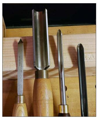
**3. Tools:** parting tool, spindle roughing gouge, detail gouge, regular spindle gouge.
