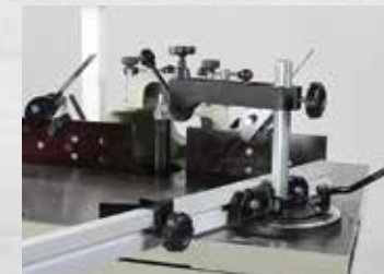
Sliding table with spindle tilt
