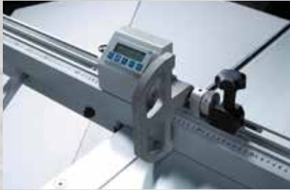
Cross cut fence w/digital readout
