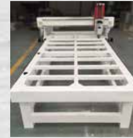
Fully welded frame
