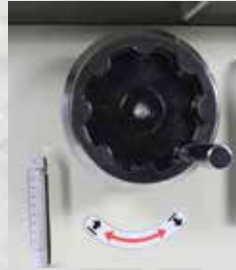
Easy spindle height adjustment
