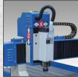
Air cooled spindle
