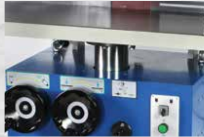
Heavy duty table lifting system
