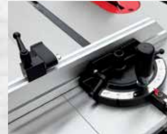
Miter fence extension with flip stop
