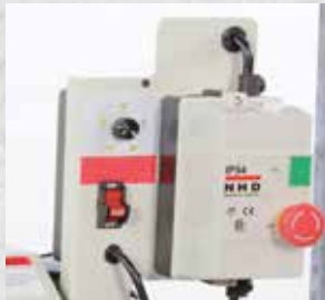
Conveyor speed control
