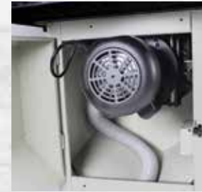
5 Hp motor with dust extraction tube
