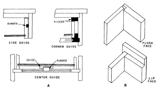
Figure 3-74.-Types of drawer guides (view A) and faces (view B).
