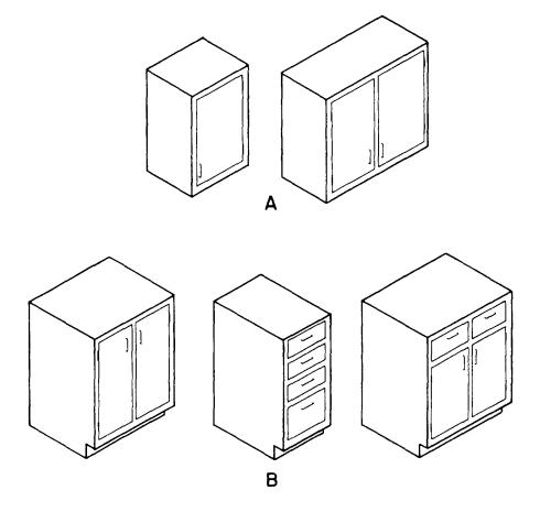
Figure 3-68.-Typical kitchen cabinets: wall (view A) and base (view B).
