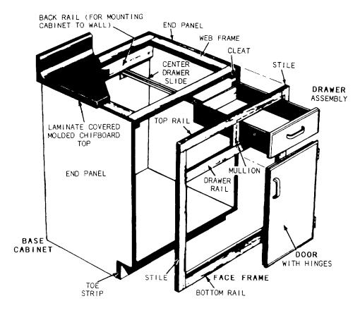
Figure 3-69.-Typical frame construction of a cabinet.
