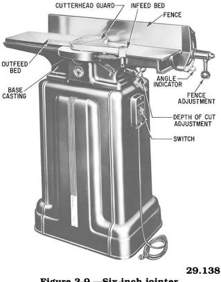
Figure 3-9.—Six-inch jointer.
