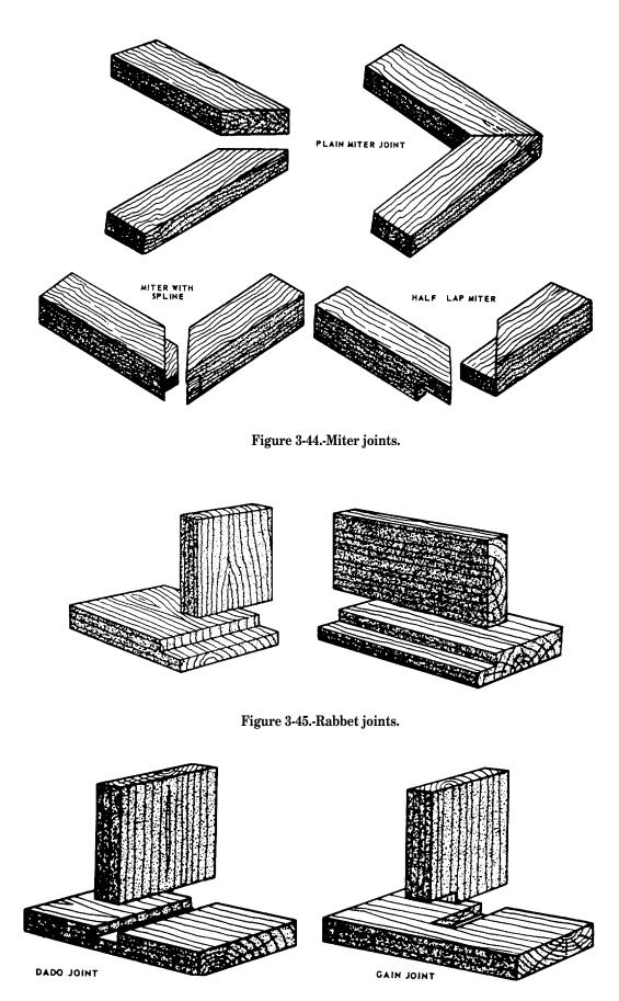
Figure 3-46.-Dado and gain joints.
