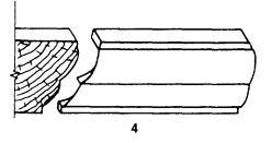
Figure 3-65.-Making a coping Joint.
