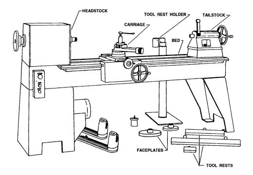
Figure 3-5.—A woodworking lathe with accessories.
