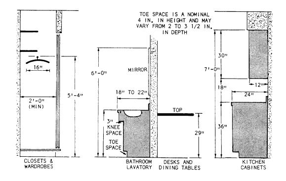
Figure 3-67.-Typical dimensions for cabinetwork.
