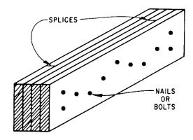
Figure 3-30.-Built-up beam.
