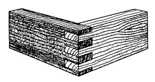
Figure 3-48.-BOX corner joint.
