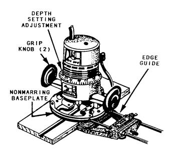
Figure 3-21.-Portable router with edge guide.
