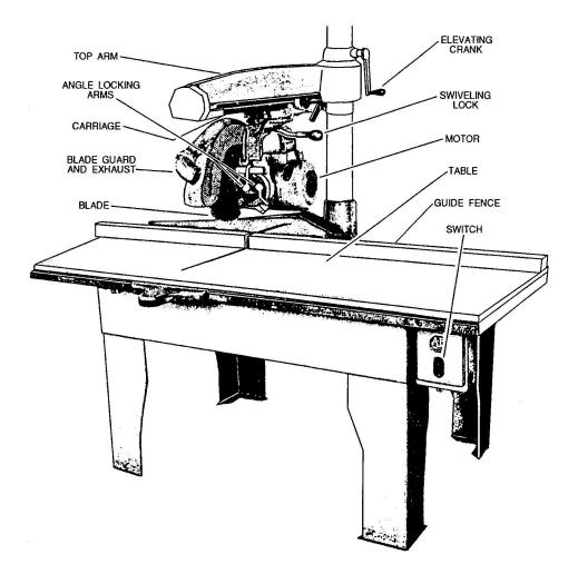
Figure 3-1.—A shop radial arm saw.
