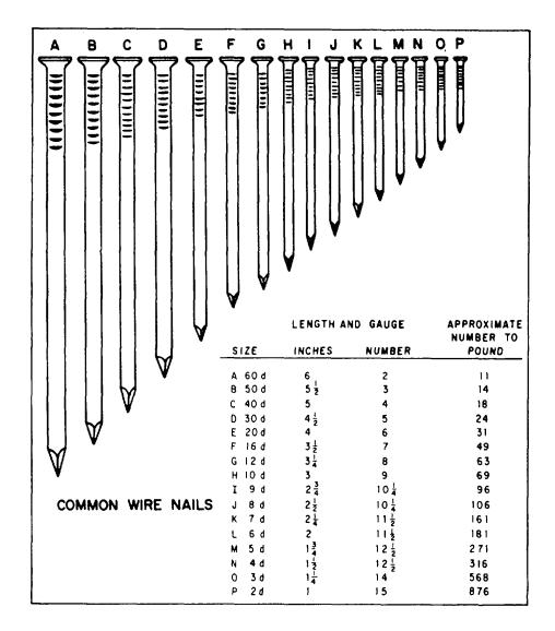
Figure 3-76.-Nail sizes given in "penny" (d) units.
