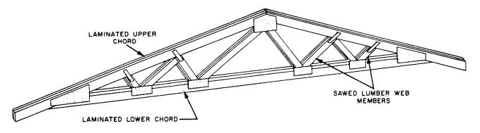
Figure 3-31.-Truss using laminated and sawed lumber.
