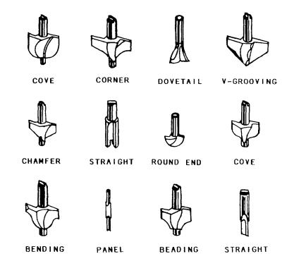
Figure 3-22.-Router bits.
