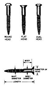
Figure 3-81.-Types and nomenclature of wood screws.
