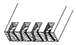
Figure 3-64.-Chiseling out waste in a through-multipledovetail joint.
