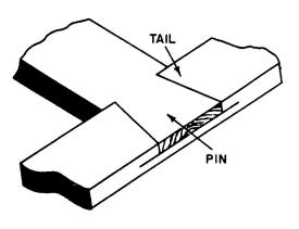
Figure 3-60.-Dovetail half-lap Joint.
