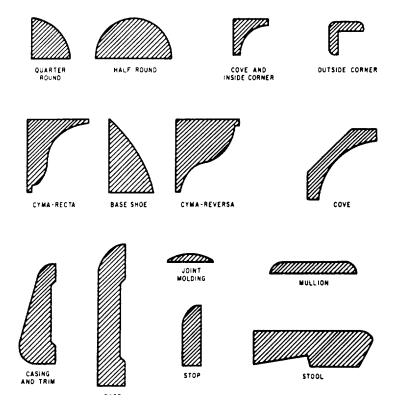
Figure 3-66.-Simple molding and trim shapes.
