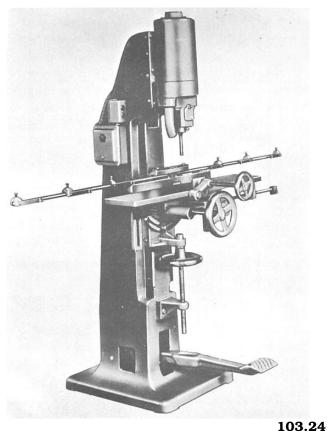
Figure 3-59.-Hollow-chisel mortising machine.
