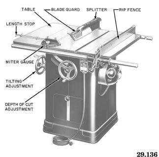
Figure 3-2.—Tilt-arbor bench saw.
