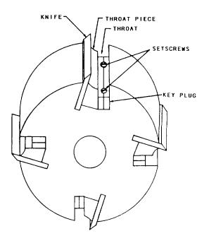
Figure 3-8.—Four-knife butterhead for a jointer.
