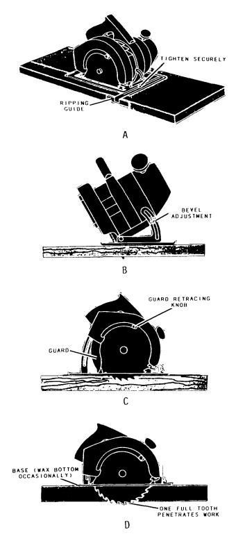
Figure 3-17.-Different ways to use a circular saw.
