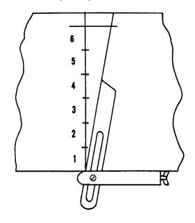
Figure 3-61.-Laying off 10° angle for dovetail joint.
