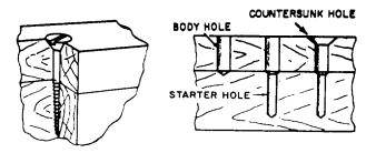
Figure 3-80.-Proper way to sink a screw.
