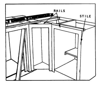
Figure 3-72.-Facing being placed on a cabinet.
