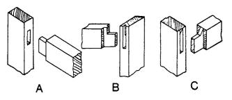
Figure 3-55.-Stub (view A), haunched (view B), and table-haunched (view C) mortise-and-tenon joints.
