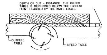
Figure 3-10.—Operating principle of a jointer.
