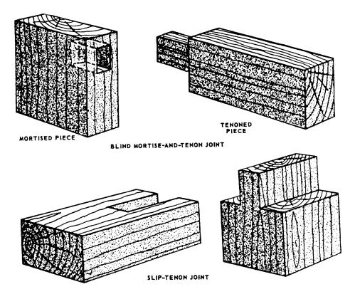
Figure 3-47.-Tenon joints.
