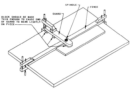
Figure 3-14.-Shaper table showing straightedge fence and guard.
