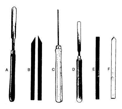
Figure 3-6.—Lathe cutting tools.
