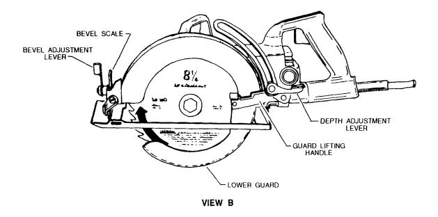
Figure 3-15.-Side-drive (view A) and worm-drive (view B) circular saws
