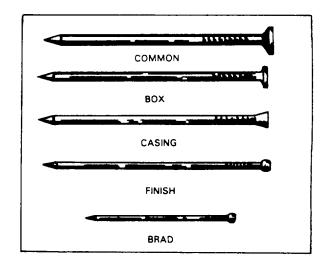
Figure 3-75.-Basic types of nails.
