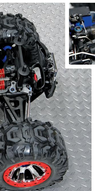
**HEAVY-DUTY DRIVESHAFTS** High-traction tires, a powerful 775 motor and locked differentials can all wreak havoc on a drivetrain. Fortunately, Traxxas is on top of things and upgraded its Revo-spec driveshafts to use a CV-style joint on both ends. The joints are supported by the full diameter of the shaft and are super smooth.
