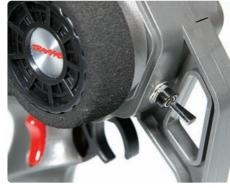
In the foreground is the three position switch to lock and unlock the diffs, and in the background you can see the bright red 2-position switch that selects high and low-range.
