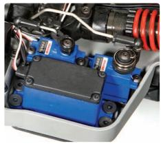
The Summit uses a total of 5 servos. Two 2075 waterproof servos for steering duties, and three 2065 sub-micro servos for shifting gears and locking the diffs.
