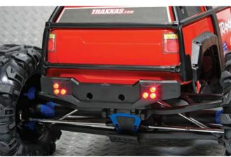
**THE LIGHTS ARE ON** The Summit comes standard with a 10 LED lighting system, so the running doesn't have to stop at dusk. The lights are always on and get power from a spare channel on the receiver. There are four bright white LEDs in the front of the truck's bumper and six red LEDs in the rear bumper. The bumpers are mounted on the chassis, so when you take the body off, you don't have to disconnect the lights.
