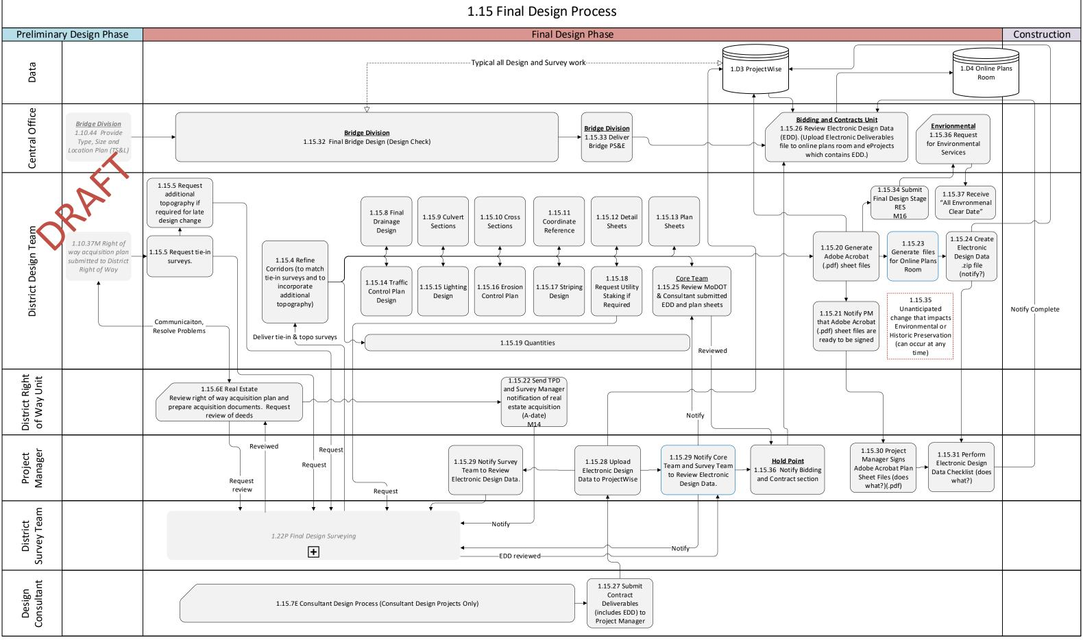
The Design Team is notified by the Survey Team when survey deliverables are updated. Likewise, the Survey Team is notified by the Design Team when any of the design data has been changed that may impact the survey workflow.
