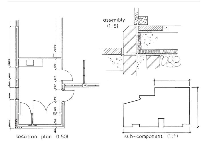
**4.2** Parts of three drawings using the Range 1 line thicknesses
