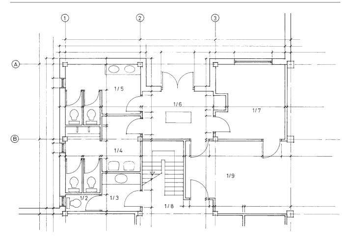
**4.15** *Typical dimensioning of general arrangement primary elements plan. (The other general arrangement plans in the set will not need to record these dimensions)*
