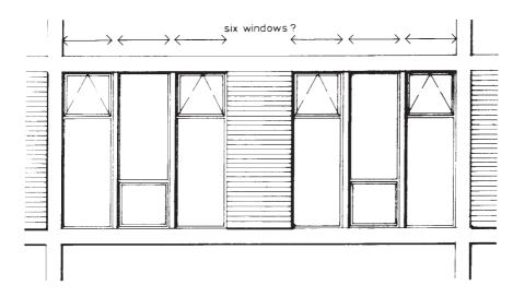
The correct procedure, however, will be to regard the whole assembly as consisting of two window components (**3.4**).
