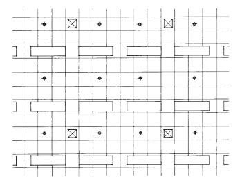
**2.10** Architect's general arrangement drawing of the ceiling finishes provides coordinating layout for everyone involved
