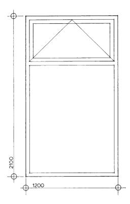
**4.14** Component destined to fill the opening shown in **4.13** is also defined by its coordinating dimension
