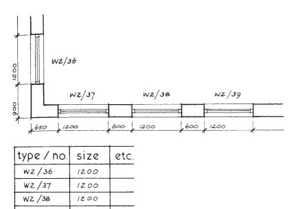
**1.6** Simple identification of components may be recorded on either a schedule or general arrangement plan
