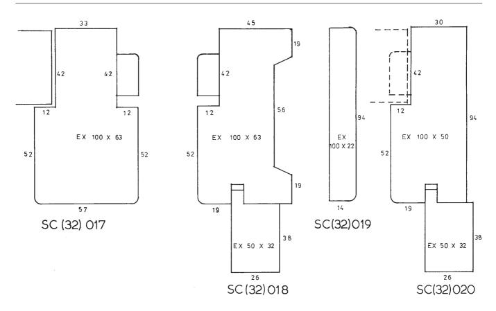
**3.10** Sub-component drawing illustrating details of the component itself. (Original scale full size)
