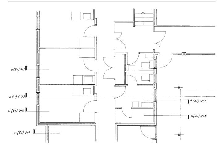
**2.21** General arrangement plans give references to general sections G(--) and strip section G(21). The former will be of the type shown in **2.19**. The latter will be similar in scope and function to **2.20**
