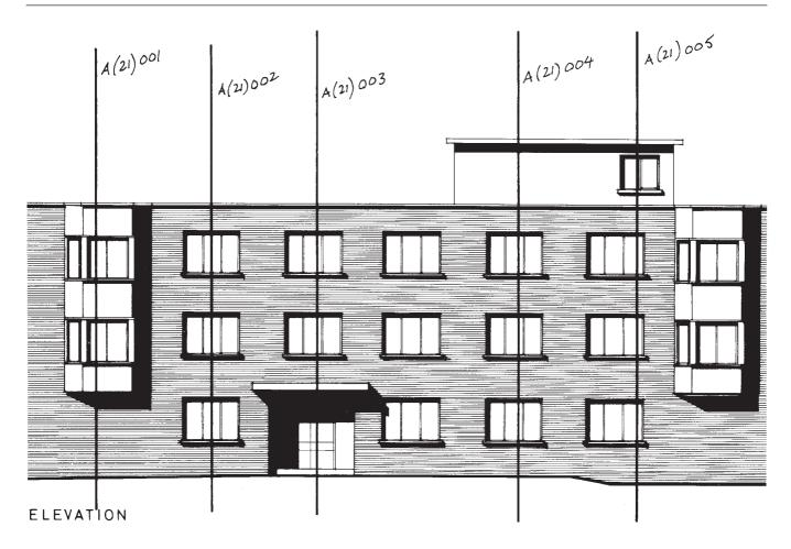
**5.7** A print of the elevation has been used to identify every section through the external walls where the construction changes
