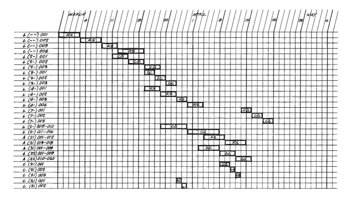
**5.14** A drawing office programme allocates individual team members appropriate work loads. The elemental approach means that DC, for example, can follow the (3-) element right through, dealing with it in its general arrangement, component and assembly aspects
