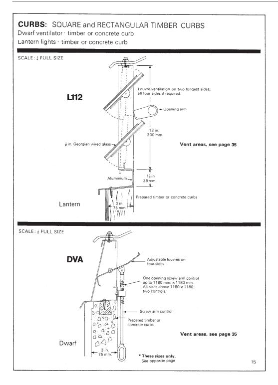
**5.4** *Manufacturer's catalogue gives precise fixing details. It is pointless to redraw this information when the catalogue can be issued to the contractor as an instruction*
