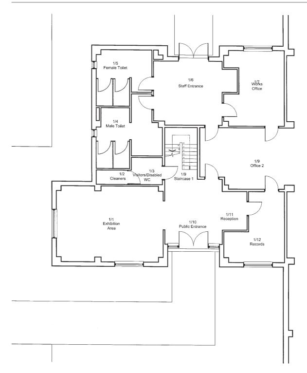
**5.2** Copy taken from **5.1** before the blandishments were added. Scale and simple draughting make it suitable for issue to consultants for preparation of their own scheme drawings (or to nominated sub-contractors when CAD is not being used)
