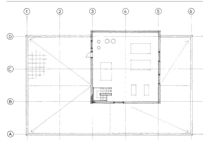
2.11 Floor plan or roof plan? The problem is avoided if all plans are treated as 'levels'
