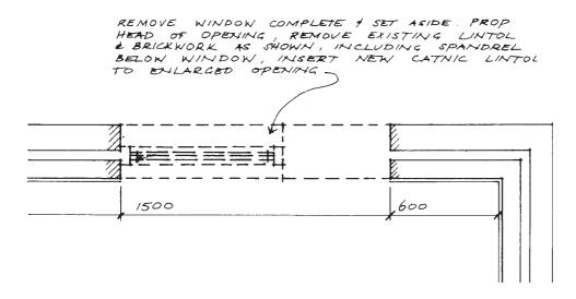
3.25 Demolition drawing covering formation of new opening in an existing wall
