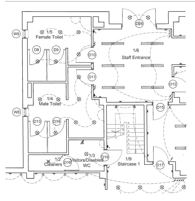
2.3 Elemental electrical layout—(63) based on 2.1
