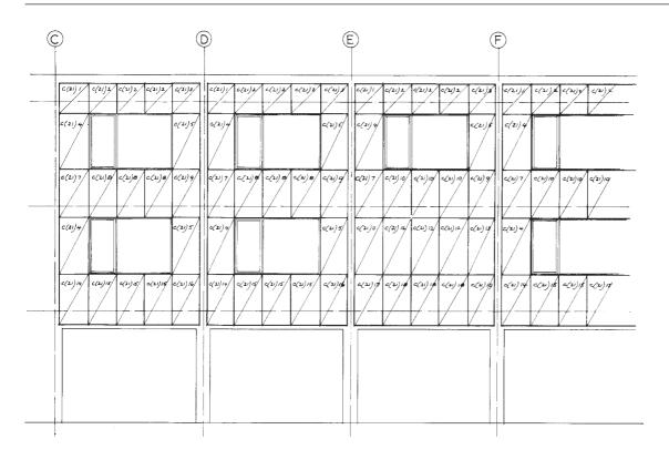
**2.17** With a limited range of panel types and with each panel's component drawing giving full information about it, the elevation itself forms an adequate schedule
