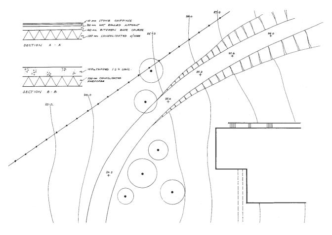
**2.23** Site plan with inset assembly details is not to be recommended. Such details form no part of what is essentially a general arrangement drawing
