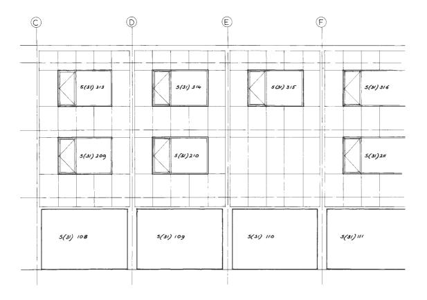
**2.16** Elevation as a secondary reference to window components. The reference S/31 leads back to the external seconday elements schedule, where the components are listed and classified
