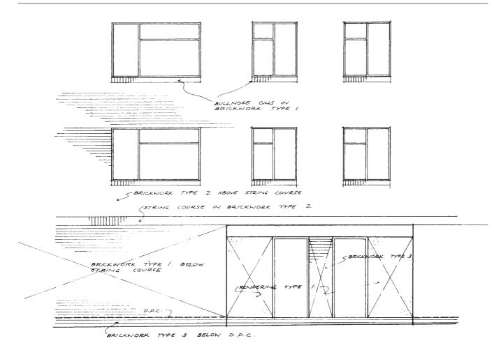
2.14 Elevations as a guide to external finishes not readily described in detail by other means
