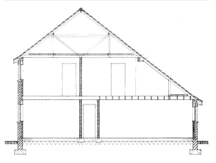
**3.16** Old-fashioned section through entire building. Far too detailed for its role of conveying information about the form and nature of the building; insufficient for anyone to build from it with confidence
