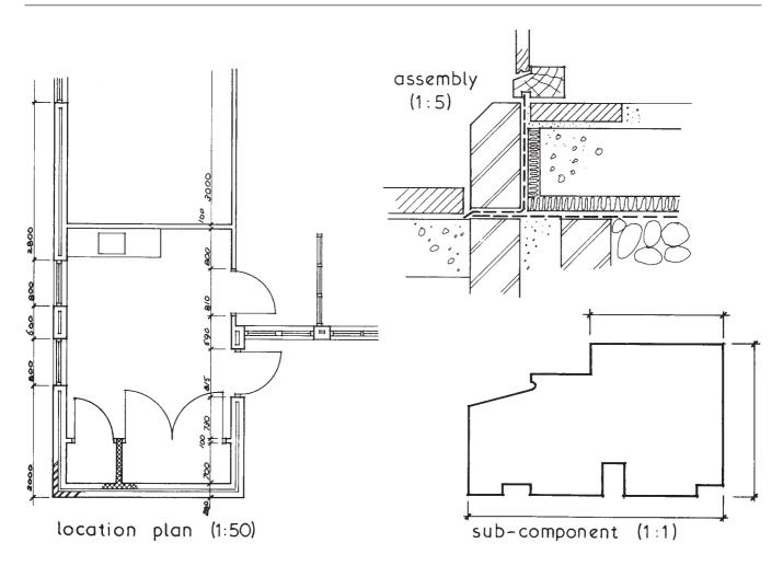
4.3 The drawing shown in 4.2 redrawn using the recommended Range 2 line thicknesses
