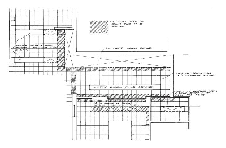
3.27 Demolition drawing of reflected ceiling plan
