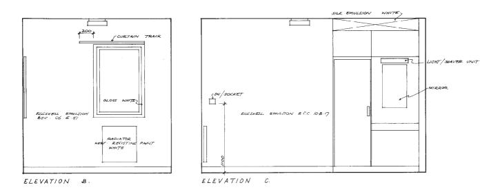
2.6 Internal elevations on a room-by-room basis is the most flexible method for conveying information on finishes (cont.)
