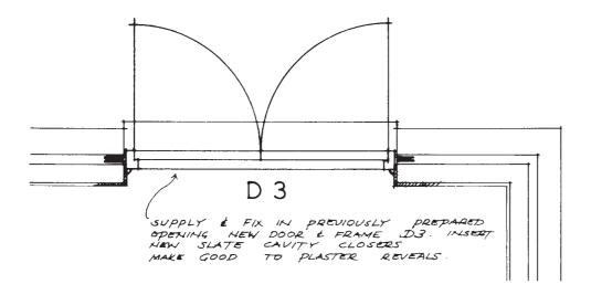
3.26 Drawing covering installation of door and frame in the opening formed in 3.25
