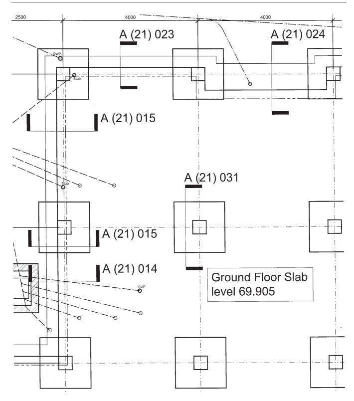
2.2 Elemental structural layout (28) based on 2.1
