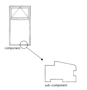
**1.10** The sub-component drawing illustrates how the component itself is made
