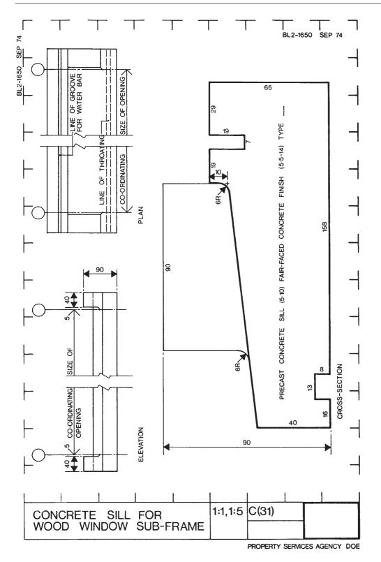
**<sup>3.8</sup>** Component detail of concrete sill
