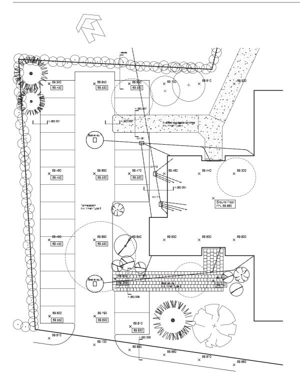
**2.22** A typical site plan. Information is given about new and existing levels as well as directions as to where other information may be found. (The information about levels is given here because the plan is to a sufficiently large scale and the small amount of earth moving makes it unlikely to form a separate contract—a good example of common sense prevailing over a more rigidly doctrinaire approach)
