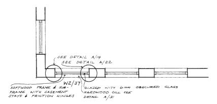
**1.7** The general arrangement plan is an inappropriate medium for recording the diverse characteristics of each component. Detail of this order can only be given elsewhere—in a specification or in other drawings to which the schedule points the way
