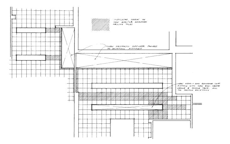
3.28 Drawing showing new works replacing demolitions shown in 3.27
