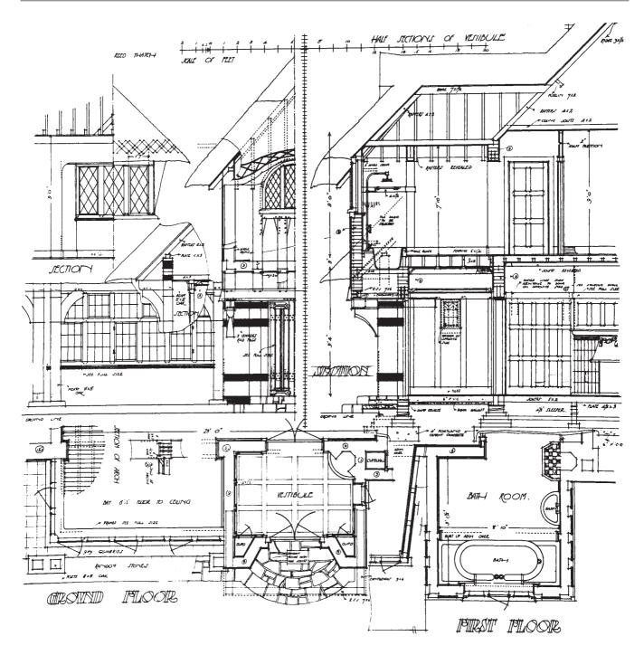
**1.2** House at Gerrards Cross by A. Jessop Hardwick, c. 1905. A typical working drawing of its era, in both its draughting techniques and its obsessive use of every inch of the drawing sheet (RIBA Drawings Collection)
