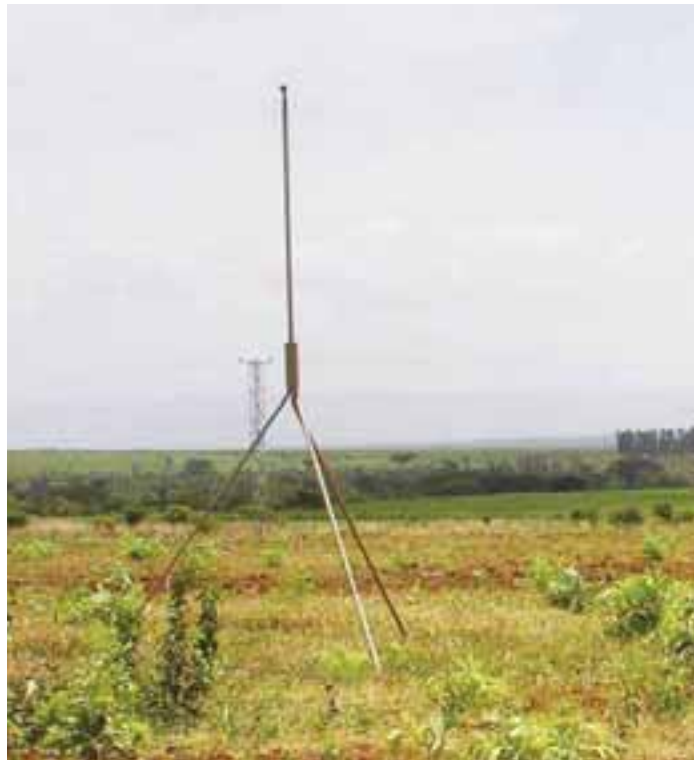
Figure 44. Movable sprinklers are used to irrigate sugarcane in Finchaa Valley.
