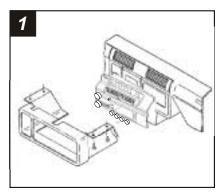
Disconnect the negative battery terminal to prevent an accidental short circuit. Remove (1) 9/32" hex-head screw from the computer diagnostic plug and twist to access (1) 9/32" screw on the trim panel. Remove (3) 9/32" screws from the bottom edge of the panel and remove. Open the glove box and remove (4) 9/32" screws from the dash trim bezel.
