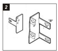
Locate **Bracket** #(L) **S-10** and the right Bracket from **Bracket Set** #5. Cut and remove all mounting tabs on the right Bracket EXCEPT top tab "B". (No cutting is required on Bracket #(L) S-10). The mounting tabs can be identified by the stamped letter on the back of each tab. Skip to the Installation Instructions for ALL VEHICLES on Page #11.
