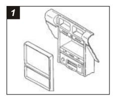
Disconnect the negative battery terminal to prevent an accidental short circuit. Using a panel removal tool, carefully pry out on the dash trim bezel and remove. Remove (2) screws securing the factory head unit and disconnect the wiring.
