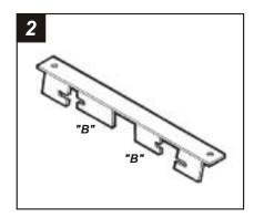
Cut and remove all mounting tabs on *Bracket Set #3* EXCEPT tabs "B". The mounting tabs can be identified by the stamped letter on the back of each tab. *Skip to the Installation Instructions for ALL VEHICLES on Page #11.*
