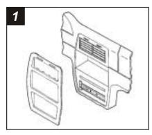
Disconnect the negative battery terminal to prevent an accidental short circuit. Gently unclip the dash trim bezel. Remove (2) screws from the factory head unit and disconnect the wiring.
