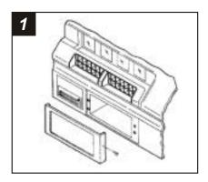
Disconnect the negative battery terminal to prevent an accidental short circuit. Open the glove box and remove (1) screw from the side of the radio trim bezel. Gently remove the bezel from the dash and the dummy plate from the bezel.
