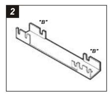
Cut and remove all mounting tabs on **Bracket #6** EXCEPT tabs **"B"**. The mounting tabs can be identified by the stamped letter on the back of each tab. **Skip** to the **Installation Instructions** for **ALL VEHICLES** on **Page #11**.
