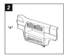
Cut and remove all mounting tabs on **Bracket #6** EXCEPT tabs **"A"**. The mounting tabs can be identified by the stamped letter on the back of each tab. **Skip** to the **Installation Instructions** for **ALL VEHICLES** on **Page** #11.
