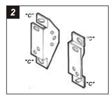
Cut and remove all mounting tabs on **Bracket Set #2** EXCEPT tabs **"C"**. The mounting tabs can be identified by the stamped letter on the back of each tab. **Skip** to the Installation Instructions for ALL VEHICLES on Page #11.
