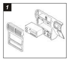
Disconnect the negative battery terminal to prevent an accidental short circuit. Using a panel removal tool, pry outward on the dash trim bezel and remove. Remove (2) screws securing the factory head unit and disconnect the wiring.
