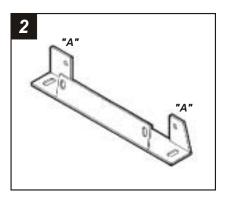
Cut and remove all mounting tabs on **Bracket #4** EXCEPT tabs **"A"**. The mounting tabs can be identified by the stamped letter on the back of each tab. **Skip** to the **Installation Instructions** for **ALL VEHICLES** on **Page** #11.
