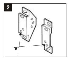
Cut and remove all mounting tabs on **Bracket Set #2** EXCEPT those tabs with holes **"B"**. The mounting tabs can be identified by the stamped letter on the back of each tab. Skip to the Installation Instructions for ALL VEHICLES on Page #11.
