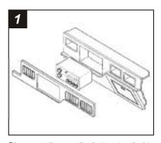
Disconnect the negative battery terminal to prevent an accidental short circuit. Remove (2) screws from the lower steering column panel. Pull the panel down to access the bottom portion of the radio trim bezel. Pull the top and bottom edges of the bezel forward and remove.
