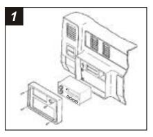
Disconnect the negative battery terminal to prevent an accidental short circuit. Remove (4) screws from the dash trim bezel. Remove the bezel and disconnect the cigarette lighter wiring.
