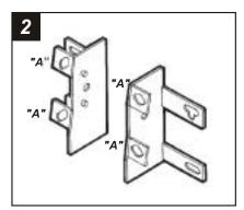
Cut and remove all mounting tabs on **Bracket #5** EXCEPT tabs **"A"**. The mounting tabs can be identified by the stamped letter on the back of each tab. *Skip to the Installation Instructions for ALL VEHICLES on Page #11*.
