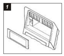
Disconnect the negative battery terminal to prevent an accidental short circuit. Carefully unsnap the radio trim bezel and remove. Remove (2) screws securing the factory head unit and disconnect the wiring.
