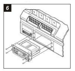
Re-connect the battery terminal and test the unit for proper operation. Mount the head unit/kit assembly to the sub-dash with those screws previously removed.
