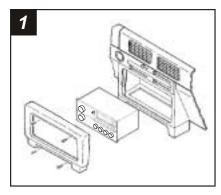
Disconnect the negative battery terminal to prevent an accidental short circuit. Remove the ashtray and (2) screws from the ashtray bracket. Remove (2) screws above the radio opening and remove the radio trim bezel.
