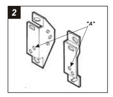
Cut and remove all mounting tabs on **Bracket Set #2** EXCEPT those tabs with holes **"A"**. The mounting tabs can be identified by the stamped letter on the back of each tab. Skip to the Installation Instructions for ALL VEHICLES on Page #11
