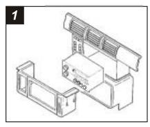
Disconnect the negative battery terminal to prevent an accidental short circuit. Remove (1) Phillips screw from each side of the center console. Open the glove box and remove (2) Phillips screws exposed. Remove (2) 7mm hex-head screws and (1) pop-clip from the lower steering column panel, and (2) Phillips screws exposed near the climate controls. Remove (1) 7mm hexhead screw under the glove box. Pull out on the center console and remove.
