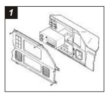
Disconnect the negative battery terminal to prevent an accidental short circuit. Remove (2) screws from the driver's side service panel and unclip the panel. Pry off the trim piece located above the glove box and remove (1) screw. Remove (3) screws from the top edge of the dash trim bezel. Remove (1) screw from the lower-left corner of the glove box and (1) screw from the parking brake release. Remove the dash trim bezel.
