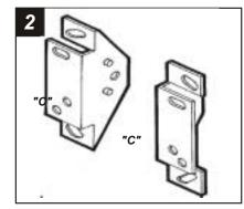
Cut and remove all mounting tabs on Bracket Set #1 EXCEPT tabs "C". The mounting tabs can be identified by the stamped letter on the back of each tab. Skip to the Installation Instructions for ALL VEHICLES on Page #11.
