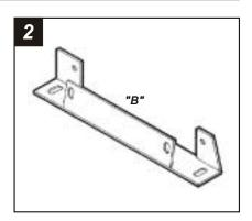
Cut and remove all mounting tabs on **Bracket #4** EXCEPT tabs **"B"**. The mounting tabs can be identified by the stamped letter on the back of each tab. Skip to the Installation Instructions for ALL VEHICLES on Page #11.
