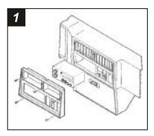
Disconnect the negative battery terminal to prevent an accidental short circuit. Remove (3) Phillips screws from the top portion of the dash trim bezel. Open the glove box and remove (2) 10mm bolts from the lower edge of the trim bezel. Pull the console trim forward and remove (2) 7mm bolts exposed. Gently unclip and remove the trim bezel. Remove (2) 7mm screws from the factory head unit and disconnect the wiring.
