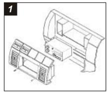
Disconnect the negative battery terminal to prevent an accidental short circuit. Remove (2) screws from the bottom of the dash trim bezel. Gently unclip and remove the bezel. Remove (4) screws from the factory head unit and disconnect the wiring.
