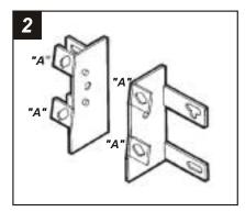
Cut and remove all mounting tabs on **Bracket Set #5** EXCEPT tabs **"A"**. The mounting tabs can be identified by the stamped letter on the back of each tab. Skip to the Installation Instructions for ALL VEHICLES on Page #11.
