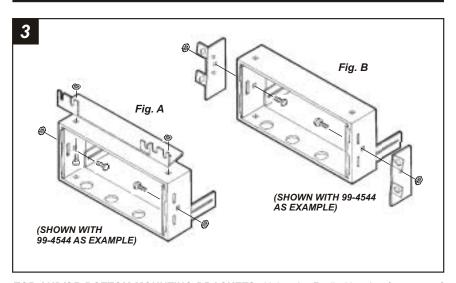
**TOP AND/OR BOTTOM MOUNTING BRACKETS:** Using the Radio Housing from one of Metra's **GENERAL MOTORS** J-body kits, secure the Mounting Bracket(s) to the Housing with Carriage Bolts and Keps Nuts. (see Fig. A)
