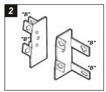
Cut and remove all mounting tabs on **Bracket Set #5** EXCEPT tabs **"B"**. The mounting tabs can be identified by the stamped letter on the back of each tab. Skip to the Installation Instructions for ALL VEHICLES on Page #11.
