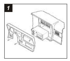
Disconnect the negative battery terminal to prevent an accidental short circuit. Remove (4) hex-head washer screws from the steering column trim panel, pull down on the rear edge of the panel and remove. Remove (4) Phillips screws from the top edge of the dash trim bezel. Remove (2) hez-head washer screws from the bottom of the dash trim bezel and remove the bezel.
