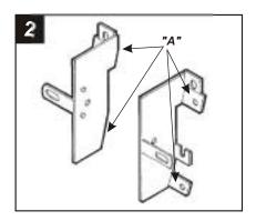
Cut and remove all mounting tabs on Bracket Set #1 EXCEPT tabs "A". The mounting tabs can be identified by the stamped letter on the back of each tab. Skip to the Installation Instructions for ALL VEHICLES on Page #11.
