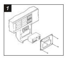
Disconnect the negative battery terminal to prevent an accidental short circuit. Remove (4) star-drive screws from the dash trim bezel and remove the bezel. Remove (4) screws securing the factory head unit and disconnect the wiring.
