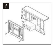
Disconnect the negative battery terminal to prevent an accidental short circuit. Remove (4) star-drive screws from the corners of the dash trim bezel. Remove (1) star-drive screw from the lower-right corner of the instrument cluster panel and remove the dash trim bezel.
