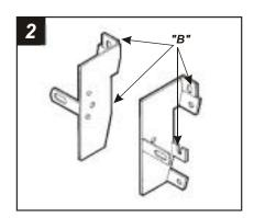
Cut and remove all mounting tabs on **Bracket Set #1** EXCEPT tabs **"B"**. The mounting tabs can be identified by the stamped letter on the back of each tab. Skip to the Installation Instructions for ALL VEHICLES on Page #11.
