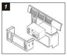
Disconnect the negative battery terminal to prevent an accidental short circuit. Remove (2) screws securing the lower steering column panel and remove. Remove (2) screws exposed on the left tab of the radio trim bezel. Open the glove box and remove (2) screws exposed on the right tabs of the radio trim bezel.
