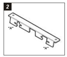
Cut and remove all mounting tabs on **Bracket #3** EXCEPT tabs **"A"**. The mounting tabs can be identified by the stamped letter on the back of each tab. Skip to the Installation Instructions for ALL VEHICLES on Page #11.
