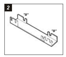
Cut and remove all mounting tabs on *Bracket Set #6* EXCEPT tabs "B". The mounting tabs can be identified by the stamped letter on the back of each tab. *Skip to the Installation Instructions for ALL VEHICLES on Page #11.*
