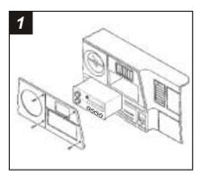
Disconnect the negative battery terminal to prevent an accidental short circuit. Remove (6) star-drive screws from the dash trim bezel and remove the bezel. Remove (2) screws from the factory head unit and disconnect the wiring.
