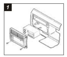
Disconnect the negative battery terminal to prevent an accidental short circuit. Remove the ashtray and (1) screw inside the ashtray cavity. Open the glove box and remove (2) screws exposed on the edge of the dash trim bezel.
